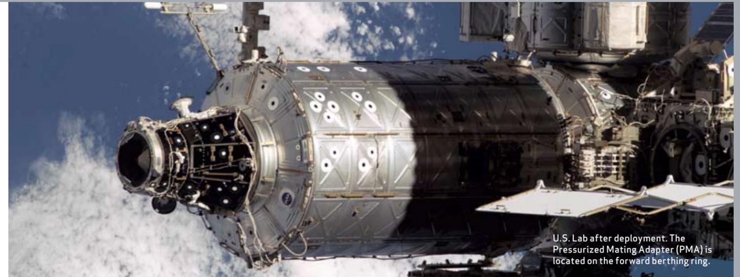
U.S. Lab after deployment. The Pressurized Mating Adapter (PMA) is located on the forward berthing ring.
