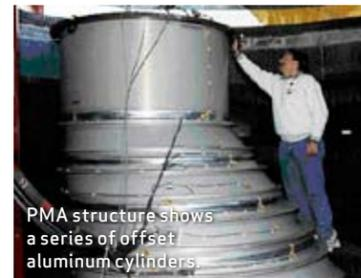
The PMA 1, 2, and 3 structures are identical and provide a pressurized interface between the U.S. and Russian ISS modules and between the U.S. modules and the Space Shuttle orbiter. The PMA structure is a truncated conical shell with a 28-inch axial offset in the diameters between the end rings.
